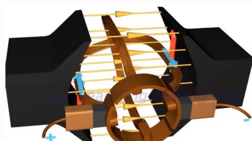
Instead of using permanent magnet, electrical magnet is used
