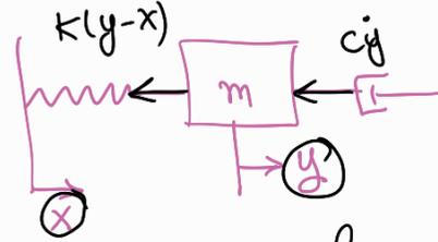
$$Kx - Ky - C\dot{y} = m\ddot{y} \quad \rightarrow \text{inertia force}$$
