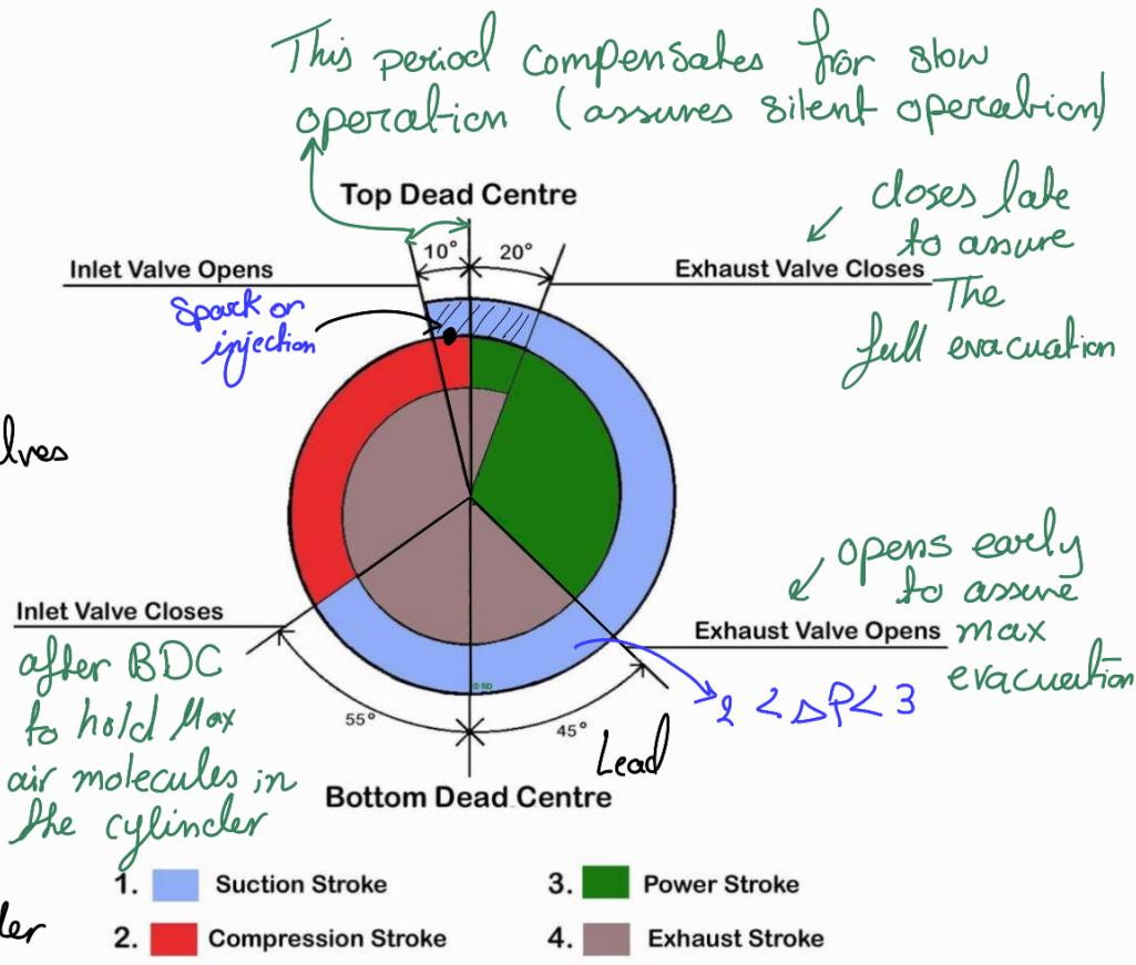
Note: In SIE over lap is larger to prevent back flow due to low pressure / Not economical at full load since unburned gases will flow pass through the engine
