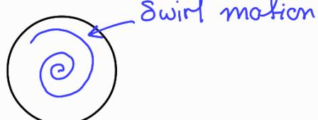
Included by swirched or masked inlet valves + Design of inlet passage
